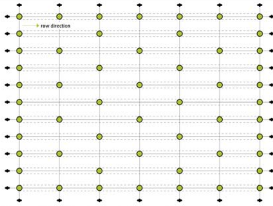
Figure 4. A possible hop yard design plan showing distribution of posts, cables, wires, stays and anchors. ● posts ◆ ground anchors - - - wire — cable
